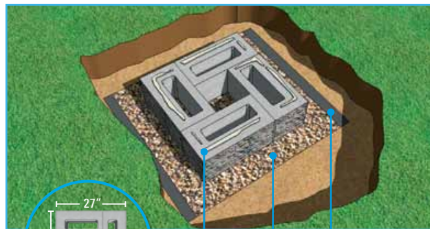
Concrete Adhesive Leveling Pad Base Stabilization Fabric
